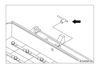
Put down the battery with fork lift or chain block by hang up hook at 4 links which located in right and left of the battery.
