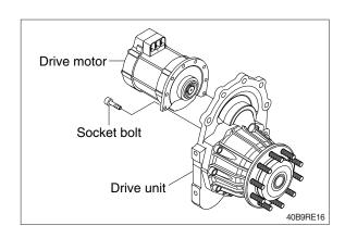
4 Loosen six mounting bolts on the truck frame and carefully take out the drive unit.
