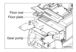
③ Disconnect the wiring of pump motor and remove the gear pump from pump motor.
