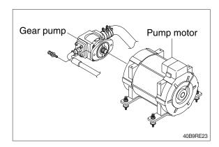
④ Remove the tightening bolts of the pump motor mounting bracket. Remove the motor from mounting bracket.
