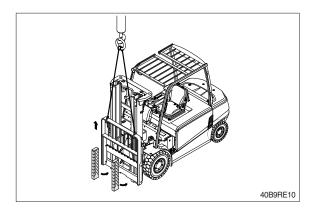
While supporting lift chains, remove the split pins and nuts from anchor pins of stationary upright.
